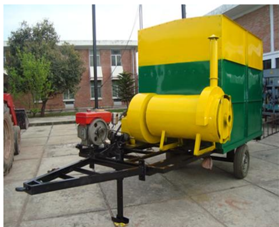
Figure 3. Experimental diesel-fired heat exchanger based turmeric dryer.
